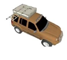
2. Open the tent by dragging the ladder, and adjust to a suitable position.
